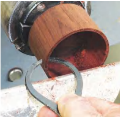
STEP 10. Accuracy rather than finish are the important things here. As you won't see the inside of the rosewood, a pair of bow leg callipers will show you if you have parallel sides
